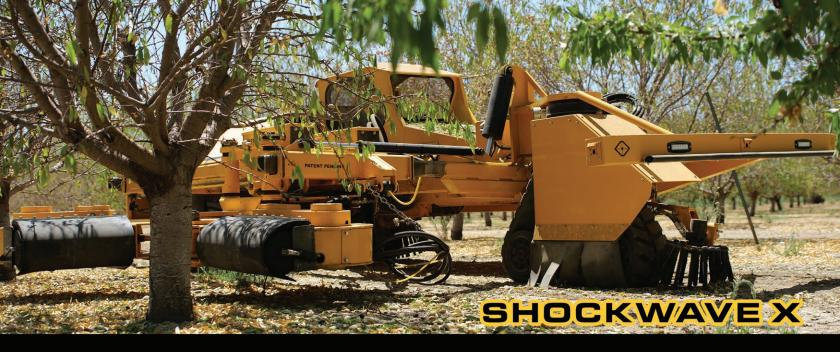
Based on our proven Shockwave Catchall X shaker frame, the Shockwave X stands apart from standard tree shakers with its constant velocity operation and 180-degree X-3 Magnum scissor grip shaker head, allowing it to slip from tree to tree with ease and precision, providing consistent results regardless of skill level.
